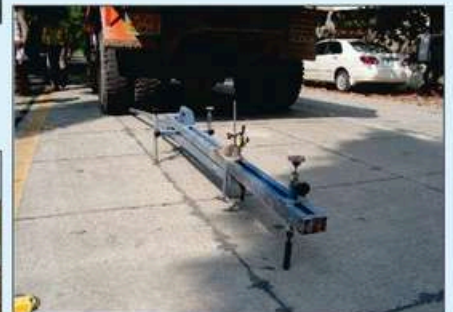
Benkelman Beam deflection Test (BBD)
