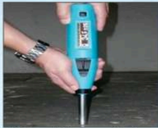
Rebound Hammer Testing
